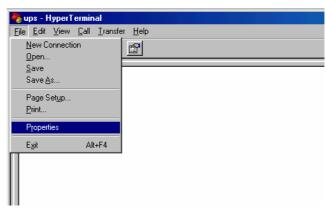
Open the Settings Tab. Function, arrow and ctrl keys act as: <u>Terminal</u> Keys, Backspace key sends: <u>Crtl+H</u>, Emulation: VT100, Telnet terminal: VT100, <u>Backscroll</u> buffer lines: 500. Click OK.
